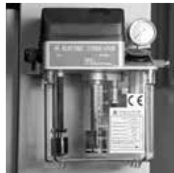
Automatic Lubrication System Otomatik yağlama sistemi
